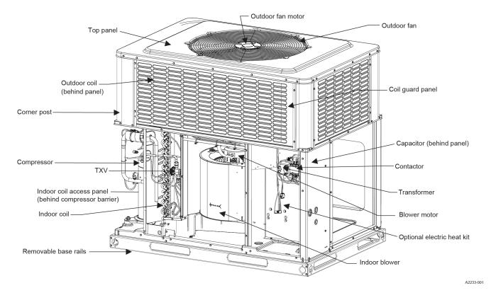
Figure 16: Unit components - PC3E48 and PC3E60 units
