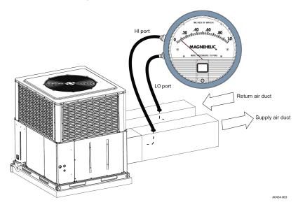
To measure the external static pressure, do the following:
