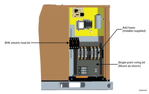
To install a single-point wiring kit, do the following:
