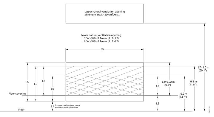
(1) **Note:** In Figure 2, only the shaded opening area below the 0.3 m point and above the floor covering (L2) counts as the effective natural ventilation area for the lower natural ventilation opening. To discern the effective natural ventilation area for the lower natural ventilation opening, you use the area between the 0.3 m point and whichever is higher of the floor covering height (L2) or the opening bottom edge height (L1).
