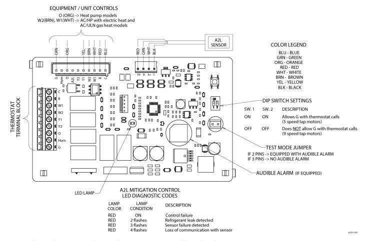
Figure 4 shows the DIP switches on the mitigation control board in the on position.
