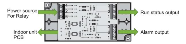
When operating RAC, Run Status signal is output When operation stops, the signal disappears. When RAC gets malfunction, alarm signal is output.
