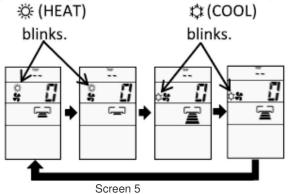
6. Press the Temperature button ( $\checkmark$  or  $\checkmark$ ) to adjust the shift value.
