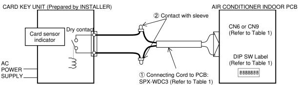
Example of wiring connection to Card Key Unit will be as below (reference only)
