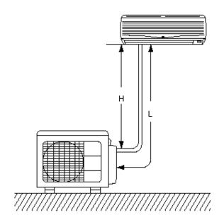
Correction Factor for **Heating Capacity** according to Piping Length
