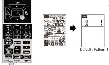
Press [ROOM TEMPERATURE setting] [\(\(UP))/[V(DOWN)] buttons. (The intermittent pattern changed with indoor unit beep sound.)
